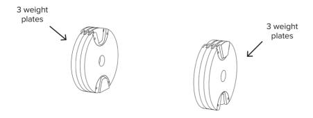
Prepare two weight stacks from the expansion kit, making sure that you have three weight plates in each stack with the hollow side of the connectors facing downwards.
