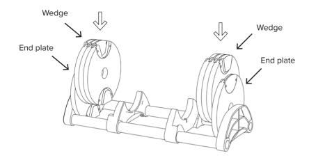
Place the weight stacks in the extended cradle, making sure that the wedge (C) on each weight stack connects to the end plate.
