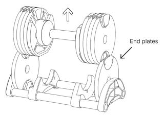
Lift the NÜOBELL and set it aside for use in step 7, making sure that only the endplates are left behind in the cradle.
