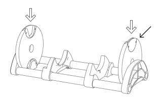
Take out the exended cradle (A) from the expansion kit and place the end plates from step 3 in their outer positions. Make sure that the flat side of the connector faces outwards.
